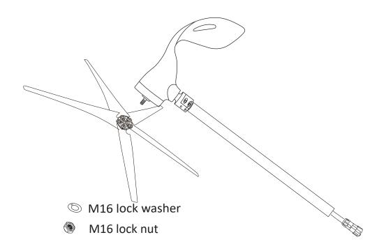
Step 7: Insert the 8mm hex key into the rotor shaft. Hold the blade assembly and tighten the M16 nut by turning the 8mm hex key counter clockwise. If needed, please use the extender (not included) to extend 8mm hex key to tighten the lock nut. Finally, spin the blades slowly to be sure they turn freely and the hub does move in along the rotor shaft.
