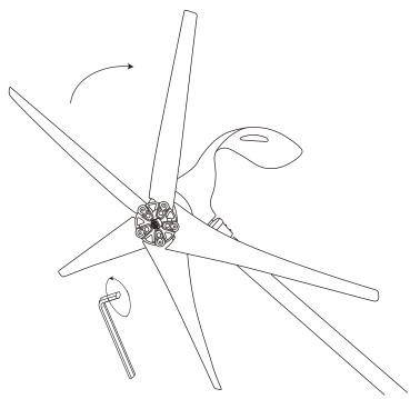
Step 8: Place the nose cone over the center line of the blade assembly and snap the nose cone into place.
