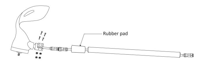
Step 4: Firmly tighten the yaw clamp bolts with the 6mm hex key. Be sure that your Nature's Generator Wind Turbine is securely attached to the pipe.
