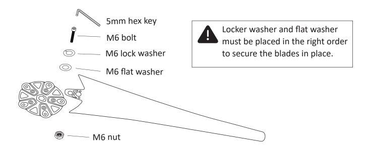
Step 6: Slide the blade assembly onto the rotor shaft and place the lock washer and lock nut on the shaft.
