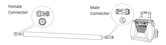
Step 2: Connect the wind turbine cable and your Nature's Generator Wind Turbine by pushing and twisting the connectors.
