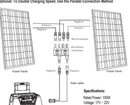
Fuse Rating: 8A Cell: Polycrystalline
