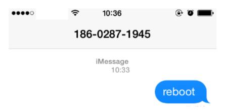
(3) In the same way, text message "cellular 1 ppp up" to make device redail-up, or text message "cellular 1 ppp down" to make device disconnect ppp connction.
