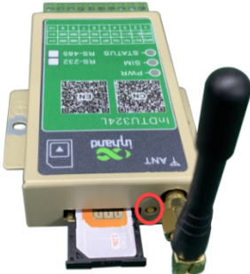
Figure 3-1-5 Installing the SIM card of the InDTU324
