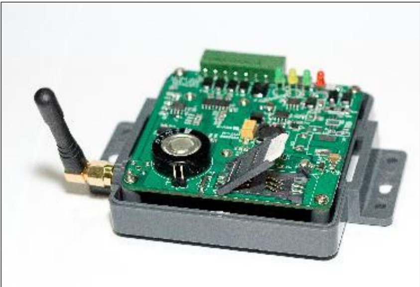
Figure 3-1-2 Installing SIM card into DTU332
