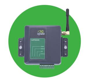
The InDTU332 series industrial grade wireless data terminal uses cellular network as the bearer network to provide wireless data transmission channel over TCP/IP. It functionally completes wireless data communications between remote control station serial devices and the central control system, to enable remote control of industrial field sites.
