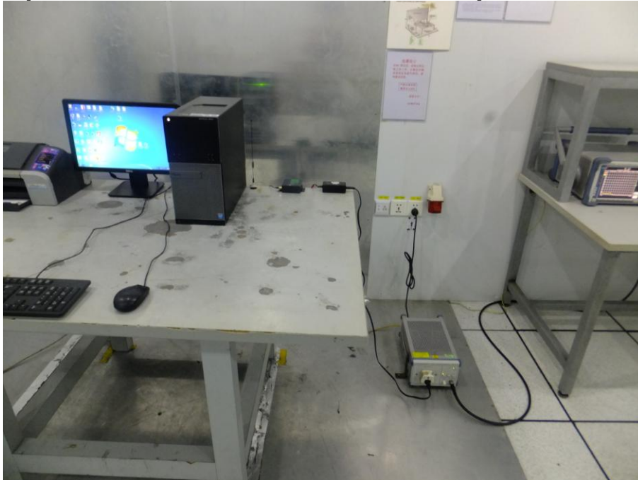
Photograph – Conducted Emission Test Setup
