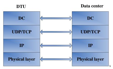
For DTU300, its physical layer is wireless cellular network, the dial link for the wireless cellular network (PPP protocol) will act as underlying bearer.
