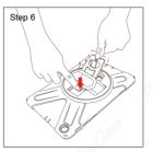
Press the button that the arrow point out ,then close the kickstand easily.
