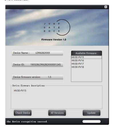
7. Choose the firmware version that you want to update (install into the Core Drive). Then click "Update" to start updating the firmware of Core Drive. (You can install any firmware version that available into your Core Drive at any time) The App will automatically download the newest firmware when the computer is connected to the internet.
