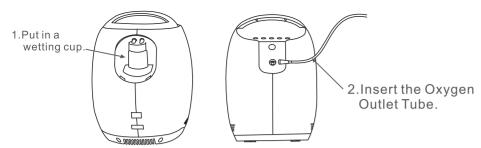
⚠ Note: The optimum installation position of the wetting cup in the machine is shown in the figure.
