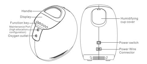
Display screen: When the oxygen generator is in operation, the display screen shows the working state of the oxygen generator.
